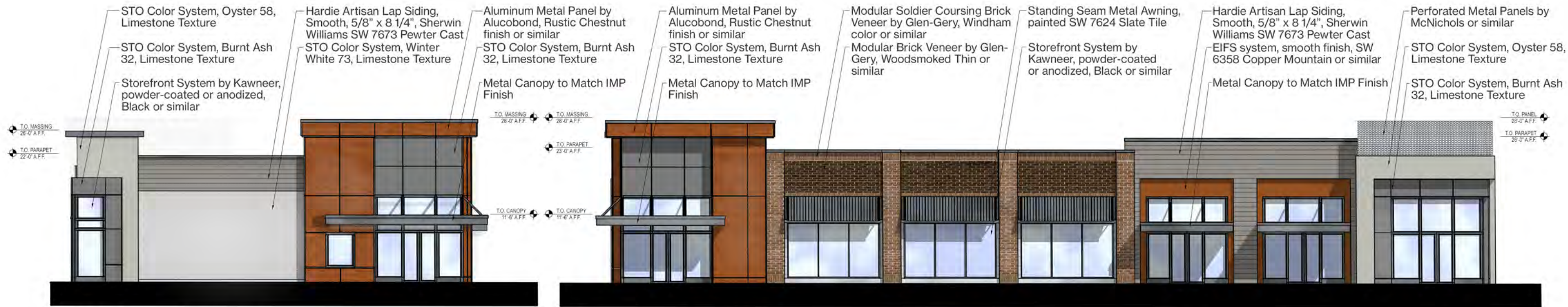
1 North Elevation (facing Parcel C) Scale: 1/8" = 1'-0"
