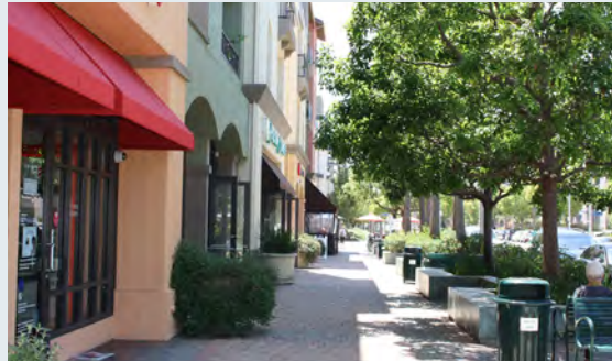
Wider walk zones of at least 7 feet are appropriate for commercial retail areas
