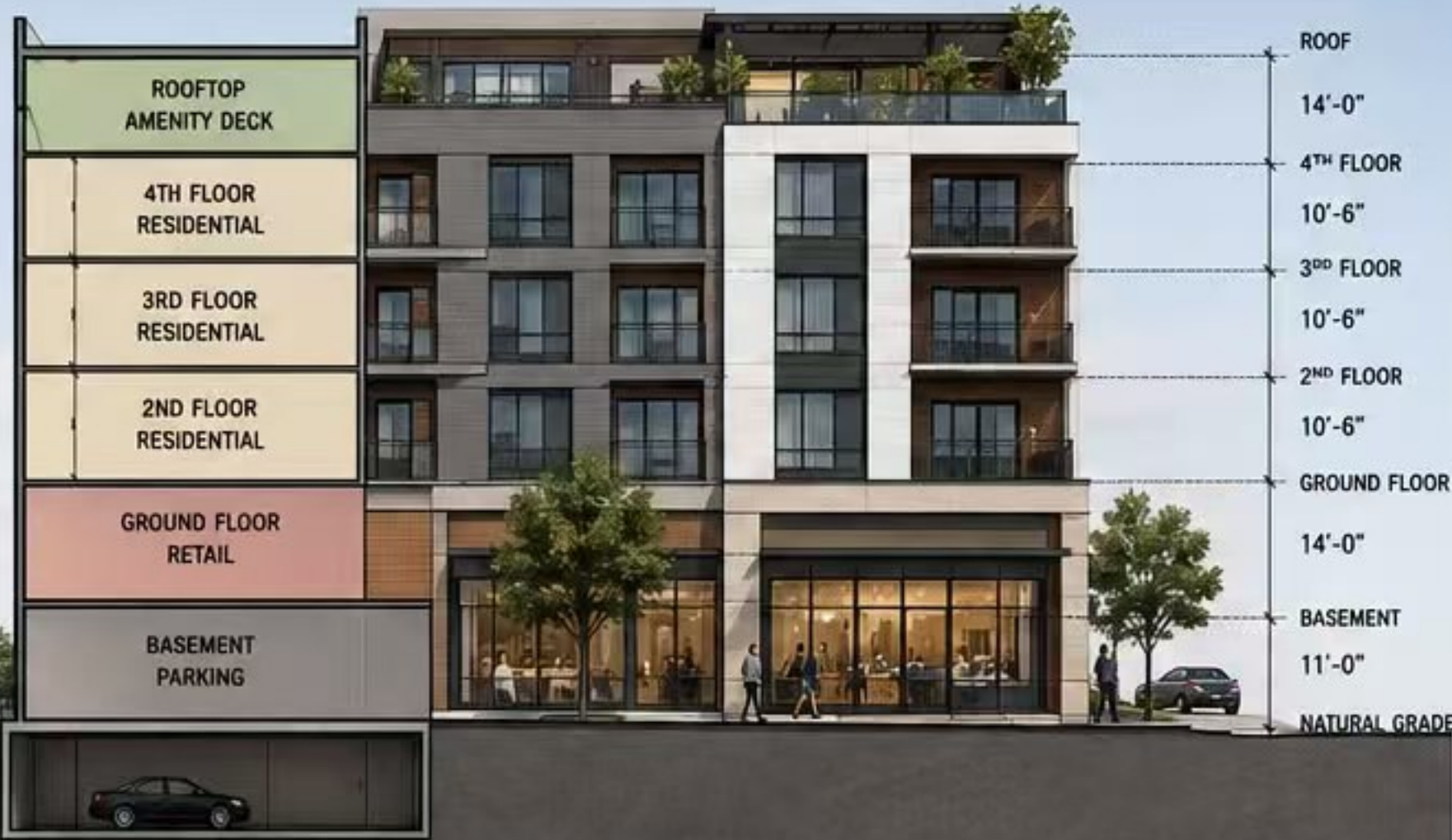
SIDE ELEVATION (NORTH VIEW)
