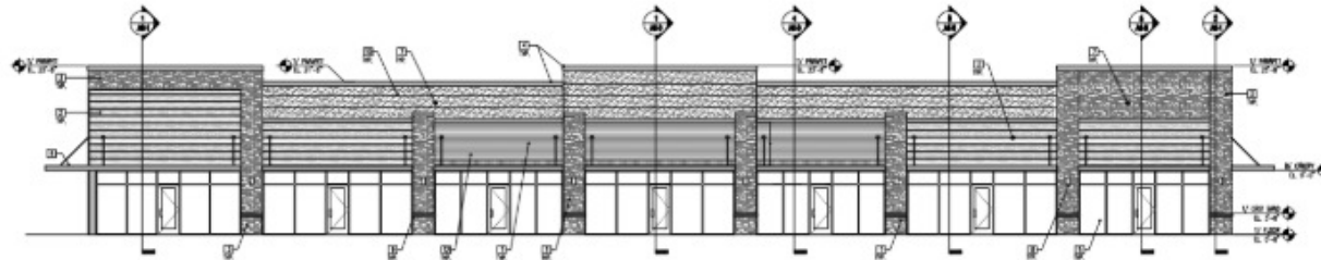
4 FRONT/SOUTH ELEVATION, BUILDING-2 SCALE 1/8" = 1'-0"
