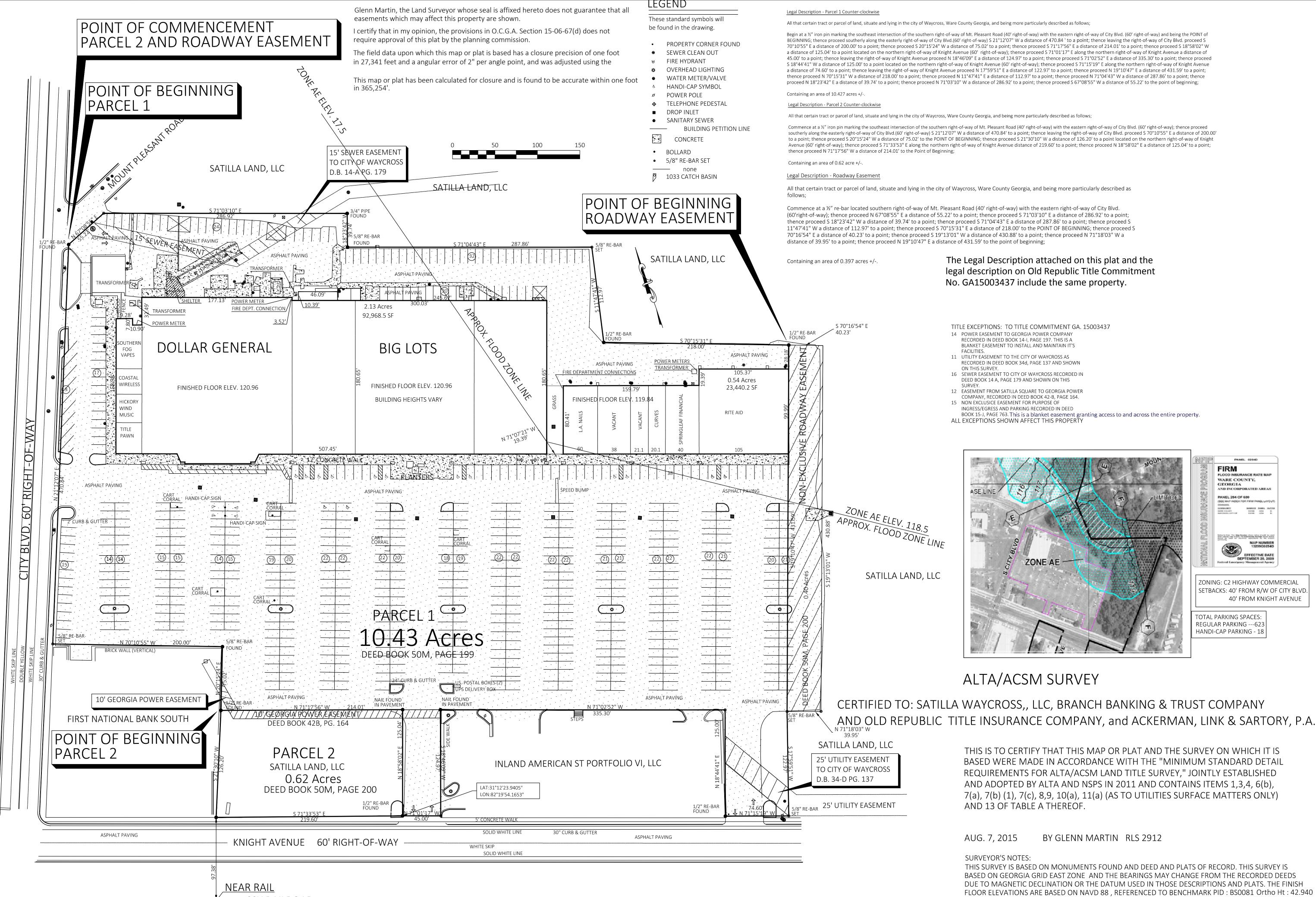
THIS SURVEY WAS PREPARED USING A TOPCON HIPER LITE + GPS SYSTEM RECEIVING NETWORK CORRECTIONS FROM EGPS GEORGIA AND A TOPCON PS103 ROBOTIC TOTAL STATION
