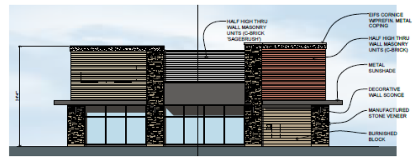
Bldg. A - East Elevation 1/8" = 1'-0"
