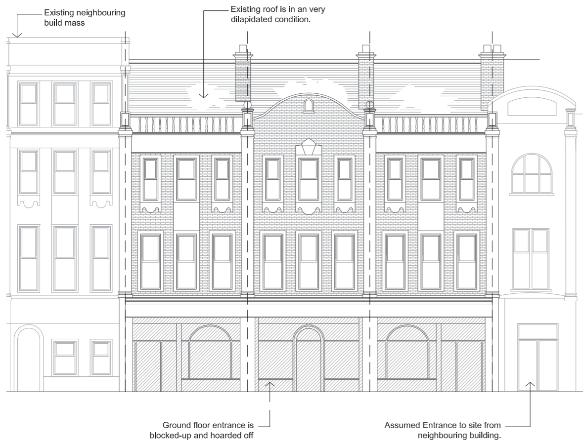
0 1 2 3 4 5 Metres Front Street Elevation
