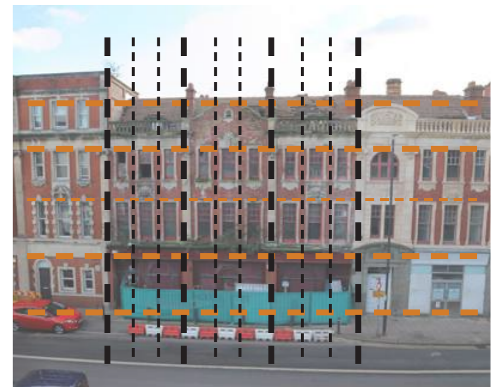
Vertical and Horizontal Elevation Grid Line
