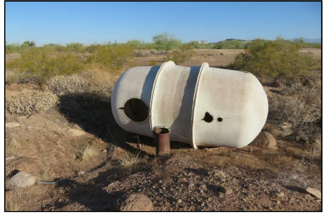
Picture 8 - A fiberglass AST (right-center) and an 8 to 10-inch diameter well casing (ADWR Well Registry No. 55-635557) on the southeast portion of the Property.
