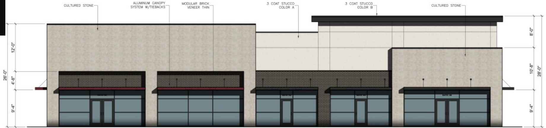
1 - (NORTH) FRONT ELEVATION SCALE 3/16"=1'-0"
