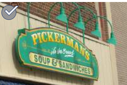
Direct lighting at signage from an external, shielded lamp.
