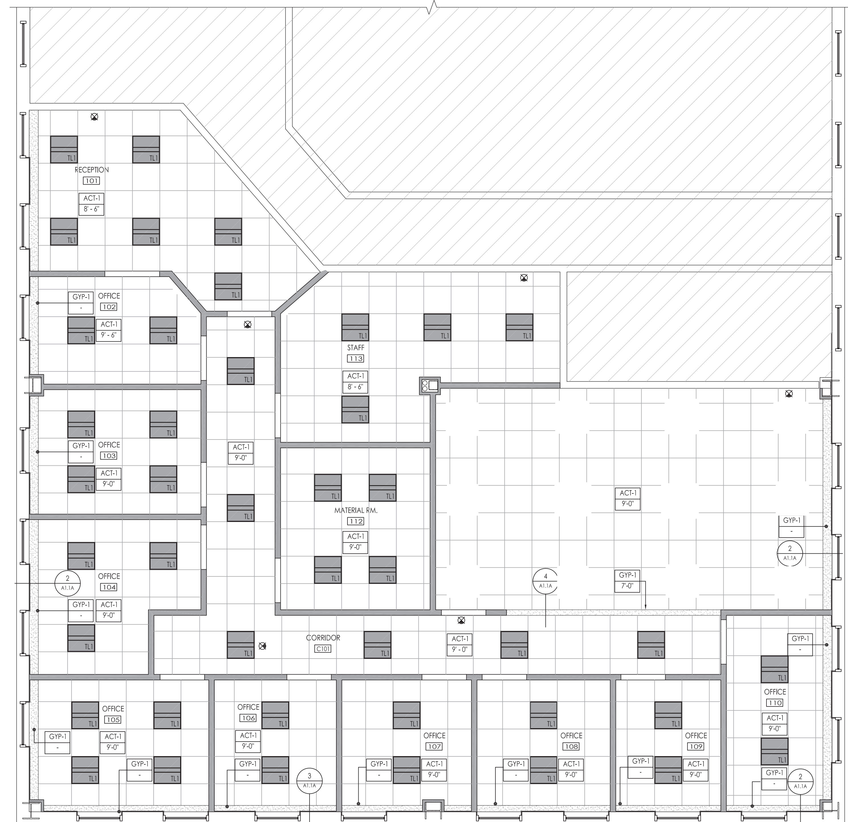
1 UNIT REFLECTED CEILING PLAN SCALE: 1/4" = 1'-0"
