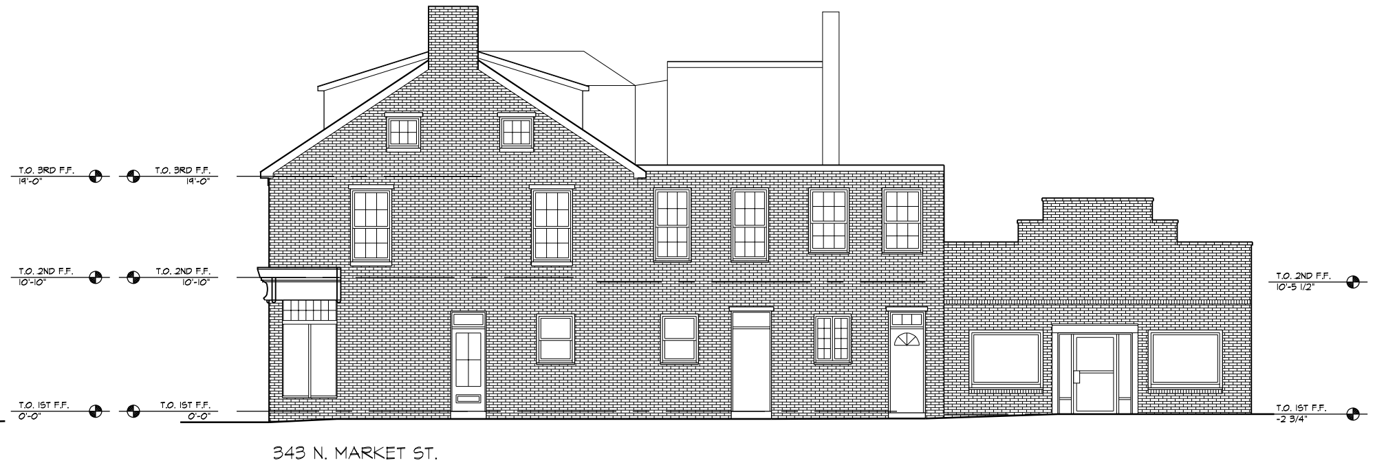
2 EXISTING FOURTH ST. ELEVATION SCALE: 3/32"=1'-0"
