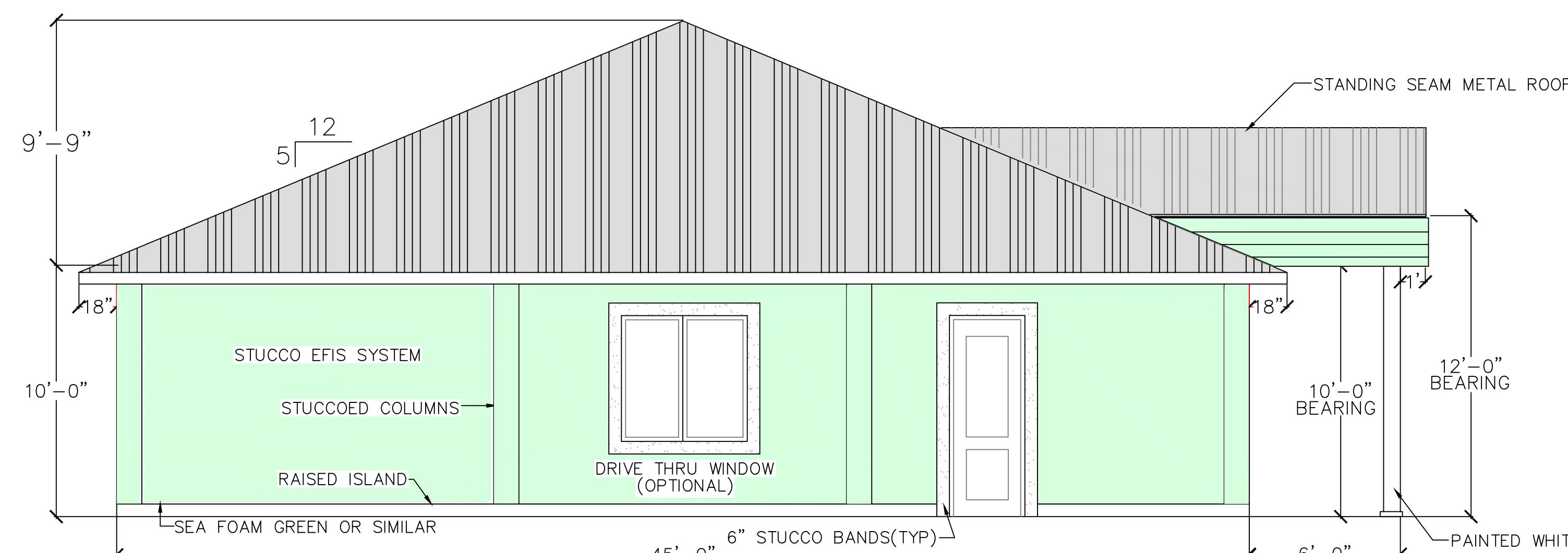
SIDE ELEVATION COVERED DRIVE THRU
