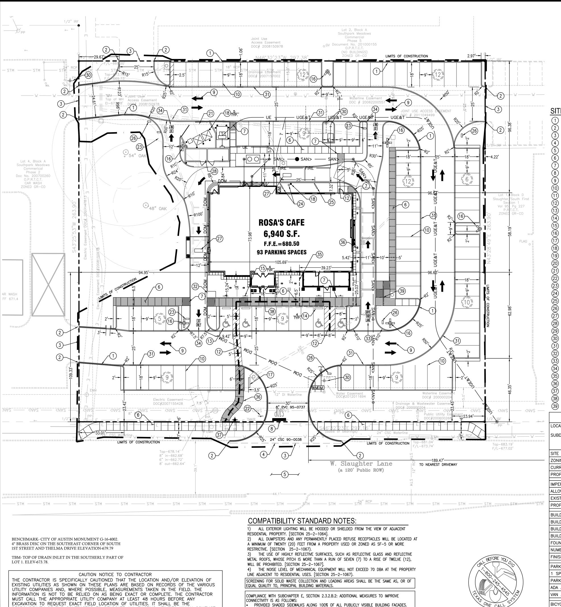
AT LEAST 50% OF PARKING AREA IS CONSTRUCTED OF CONCRETE.
