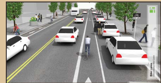
Bike Lanes: 5-6' wide. Located between driving and parking lanes. Best for streets 25-35 mph.
