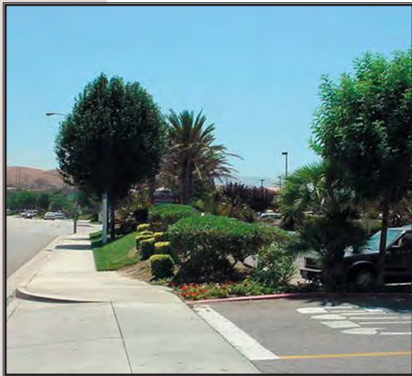
PARKING LOTS CAN ALSO BE SCREENED BY ROLLING EARTH BERMS AND CHANGES IN ELEVATION
